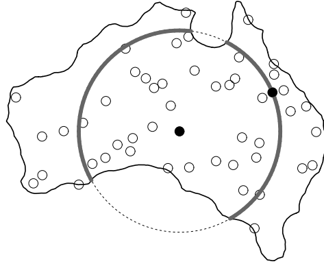
Figure 7.17. Calculation of sampling bias for the isotropic correction. The contribution from a pair of data points x_i, x_j is determined by drawing a circle through x_j centred at x_i . The fraction p of the circle's perimeter which falls inside the observation window (grey line) is measured. The edge correction weight for this pair of points is 1/p .
